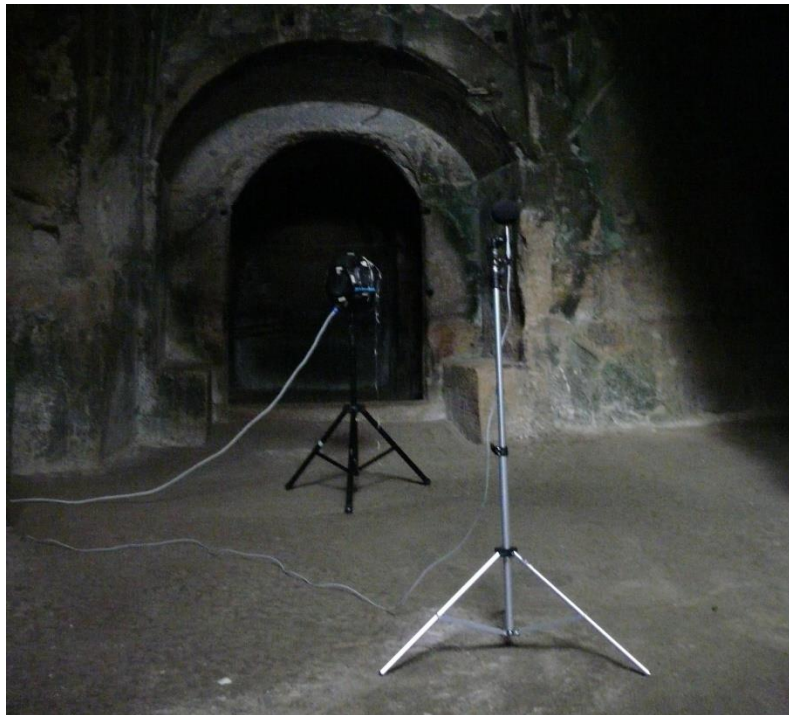
Figure 5. Sound source and microphone in the room in which lived the Sibyl.
