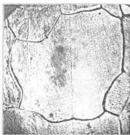
Fig. 9. Specimen after 1000 revolutions of a stress of 12.4 mm per sq inch at 1000.
