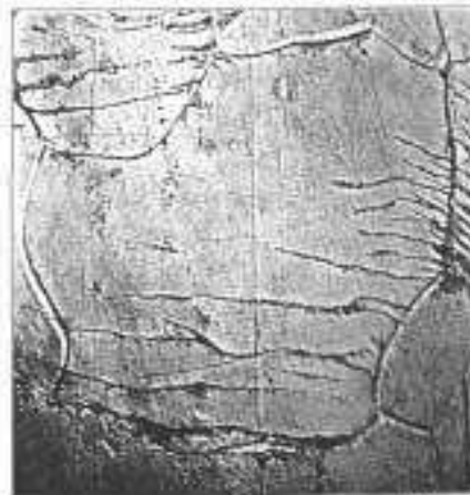
Fig. 7. Photomicrograph of the progression of cracks in a material due to fatigue
