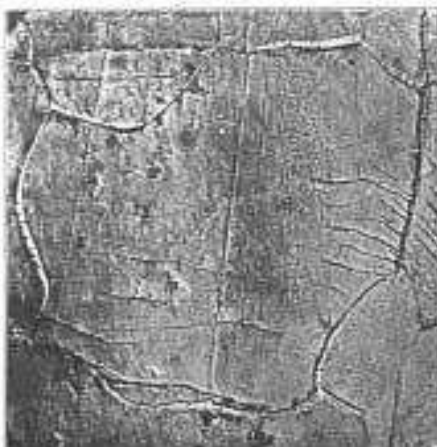
Fig. 7. Photomicrograph of the progression of cracks in a material due to fatigue
