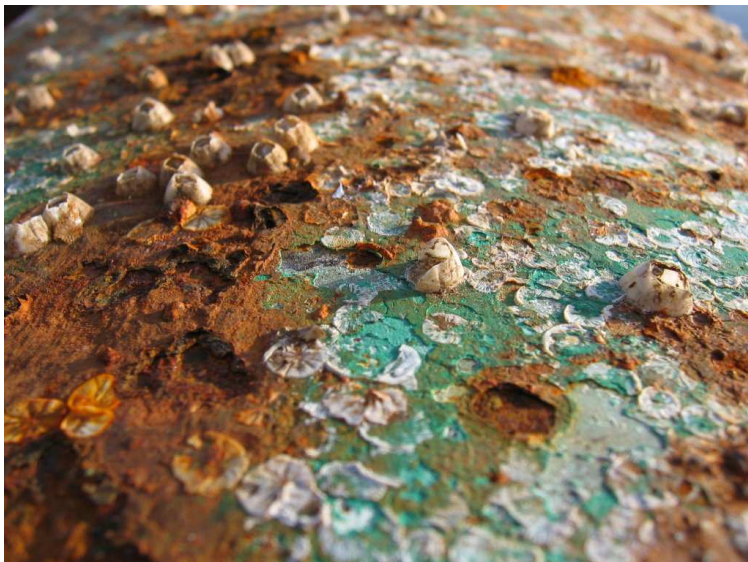
Fig. 16. Antifouling only temporarily limit the corrosion of boat hulls
